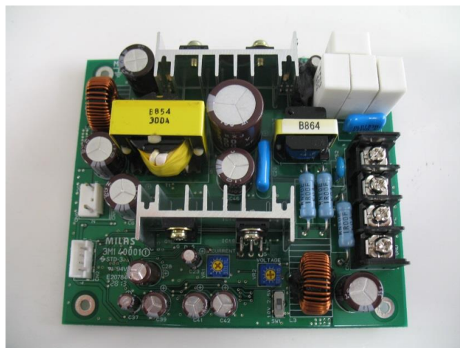
Appearance of power supply for Deuterium Lamps
